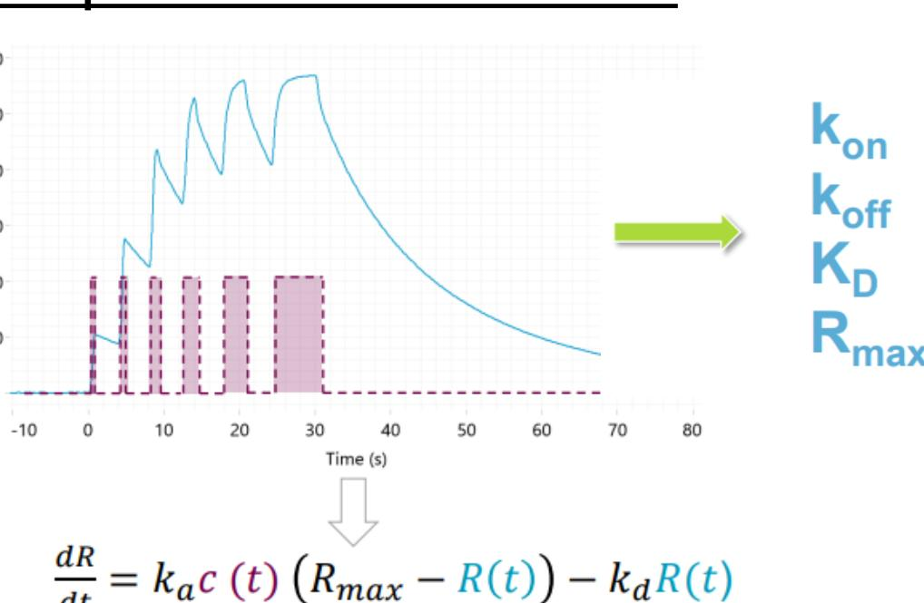
While traditional methods rely on injections of different analyte concentrations from different wells, waveRAPID uses varying injection durations from a single well to achieve a time dependent concentration function ( $c(t)$ ), which is then used in an ordinary differential equation to determine kinetic parameters
