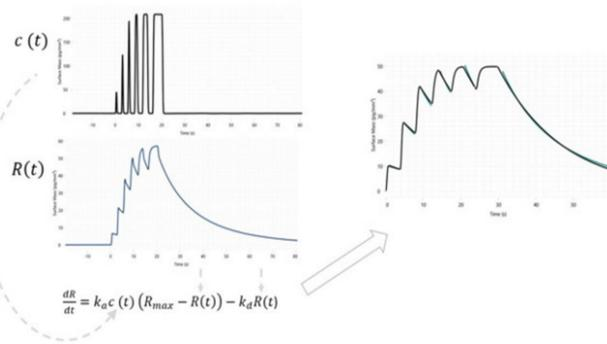
The Creoptix® wave can utilize the proprietary WaveRAPID analysis mode. In the WaveRAPID mode one analyte concentration is pulsed repeatedly with increasing duration. The time-dependent concentration function is shown at the top left, and the sensorgram response is shown at the lower left. As with a traditional kinetics approach, the
