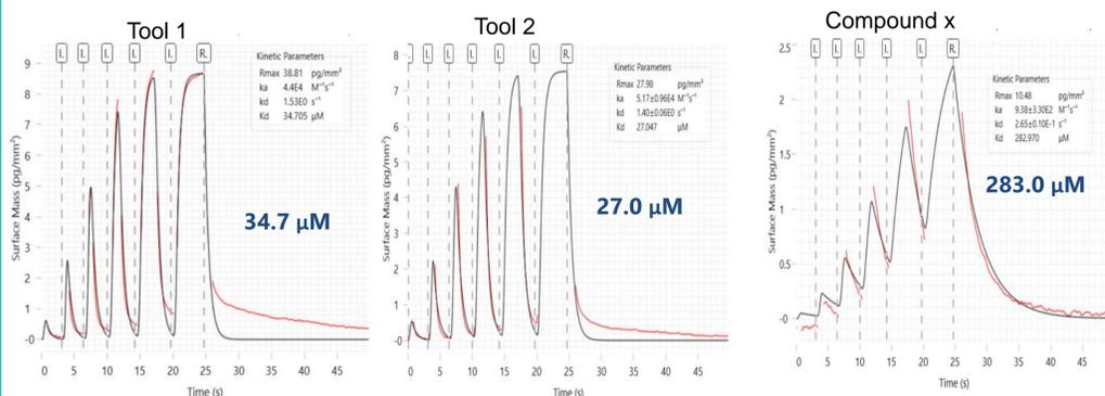
The 1:1 kinetic binding fit is the default fitting in the software and whilst the fit looks possible, the errors for Tool 1 and Tool 2 are close to 30%. Over a n=3 for each compound the  $k_a$ ,  $k_d$  and  $K_D$  values are similar, and the data is very reproducible.
