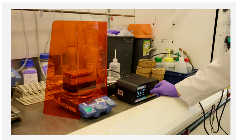
Figure 3: Lumidox II photochemistry apparatus, used here for a decarboxylative photoredox coupling reaction
