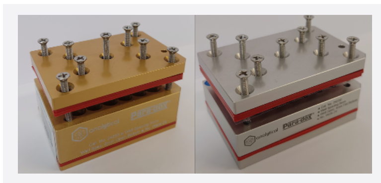
Figure 1: A 24 x 1 mL well-plate (left) and a 24 x 200 \mu\text{L} well-plate (right)
