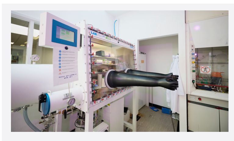
Figure 2: MBRAUN LABstar pro glovebox, used for setting up plate-based reactions
